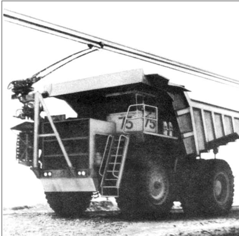
Trolley truck operating at the Quebec Cartier iron ore mine, Lac Jeannine, 1970s
