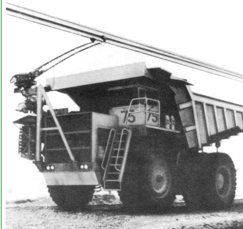
Box 15. Trolley truck operating at the Quebec Cartier iron ore mine, Lac Jeannine, 1970s
