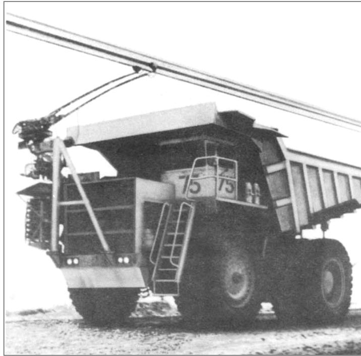
Figure 3. Trolley truck operating at the Quebec Cartier iron ore mine, Lac Jeannine, 1970s. 29
