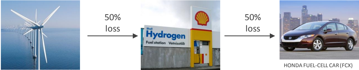
Figure 7. Comparison of the transfer of traction energy by hydrogen with transfer by electrons
